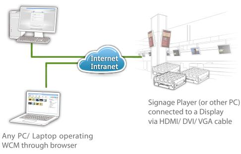
Above three components should be connected via Internet or Intranet.
